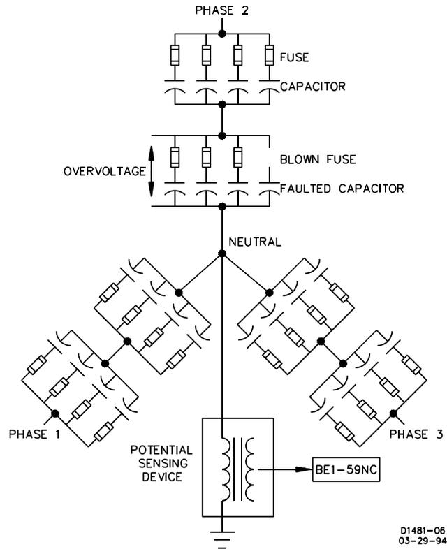
Figure 1-1. Ungrounded 3-Phase, 3-Wire System
