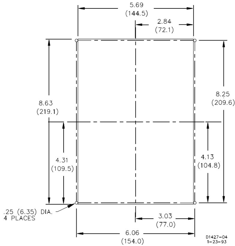
Figure 4-1. S1 Case, Panel Drilling Diagram, Semi-Flush Mounting
